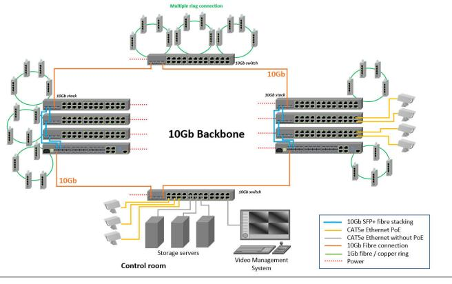
Network performance barriers are on the rise. Growing demand for bandwidth, to support high-end applications, requires the deployment of 10-Gigabit solutions.
